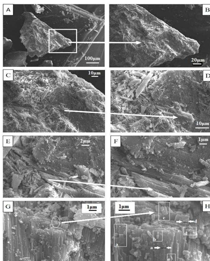
**Figure 3.** SEM images of crossed lamellar layers occurring in shell of *Eobania vermiculata*. A, B, C, D, E and F the point determined on the *E. vermiculata* shell fragment at 100, 20, 10, 2, 1 micron, respectively. G: Thin prisms from lamellar of *E. vermiculata* at 1 μm (Mag: 20.00 KX). H: Elongate, lath like, thin prisms from acrossed-lamellar layers of *E. vermiculata* at 1 μm (Mag: 40.00 KX): Cross-layered layers are 370 nm, 160 nm, 360 nm, 355 nm, 155 nm thick, respectively.
